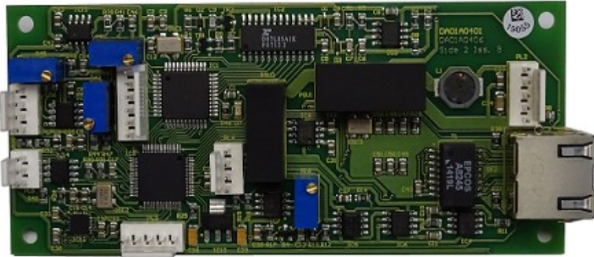
Ethernet Board Top Side
