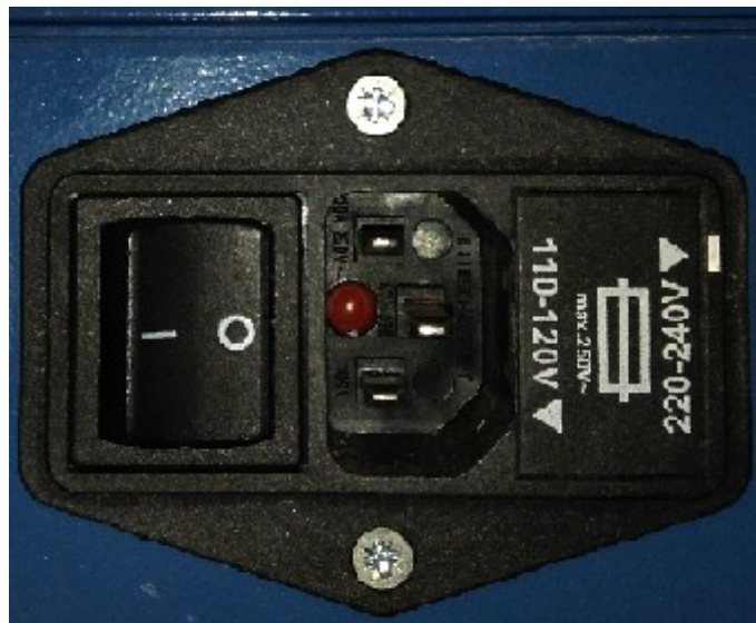
IEC Connector on back set up for a voltage input of 220 - 240V AC
